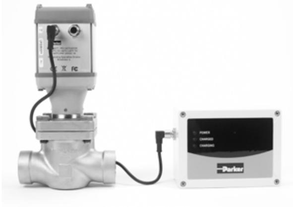
The PEV Backup Module is designed to bring the PEV electronic control valve to a user-defined position upon loss of power. The PBM can replace an upstream solenoid valve or user supplied uninterruptible power supply and offers a higher level of safety to the entire system. The PEV-PBM combination can be programmed to return to a full open, full closed, or defined position. Instructions on how to program the loss of power position see the software parameters table on page 8 (level 1; section 07).
