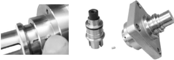
Figure 14: Removal of the PEV Plug
