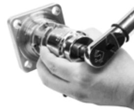
Figure 12: Removal of the PEV Seat Disc
