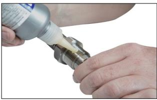
Apply liquid gasket / Teflon to the conical thread. Install the mechanical part and tighten it. Tighten depending on the thread type and size (80-150Nm).
