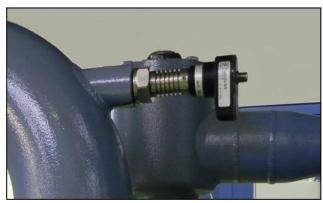
Mount the electronic part again and secure with two set screws.
