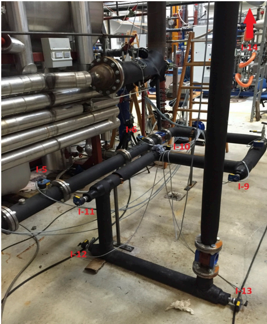
Figure 13: The sensor mounting on the Laboratory test system.
